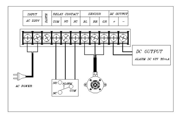
110/220 Input: To fix the power supply selection switch to AC110V or 220V and then to connect the line. (AC230V 50Hz AC110V/ 50Hz option)
