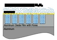
The operating principle is similar to that of other aluminum oxide sensors: a hygroscopic layer of aluminum oxide adsorbs or releases water molecules
