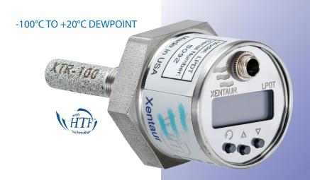
Xentaur's Model LPDT is the world's smallest loop powered (2-wire) dewpoint transmitter with a display. The compact LPDT is a fully functional instrument operated through a miniature custom LCD display and three push buttons, using the same user friendly interface of all Xentaur hygrometers. The analog output is linear to the engineering units selected for display and is user configurable. A weatherproof cap is available for outdoor NEMA 4X (IP65) applications.
